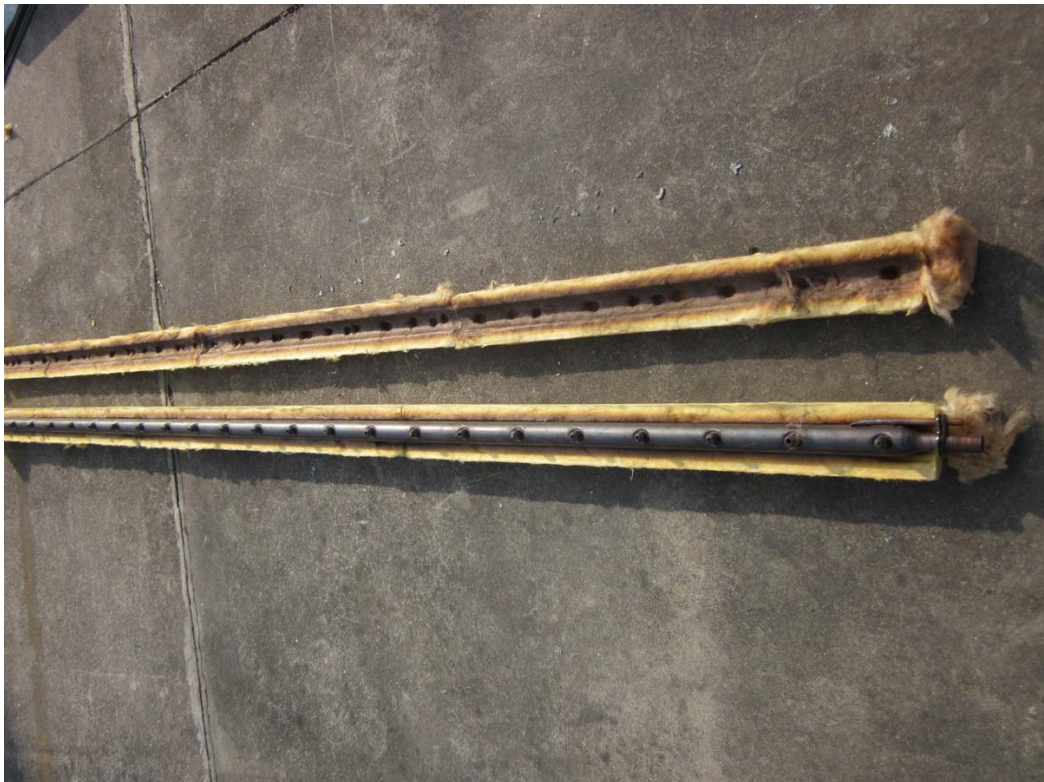
Figure C.4: Photo of the insulation (after exposure test)
